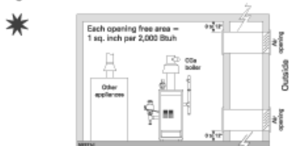
Figure 5 Air from outdoors – horizontal ducts
